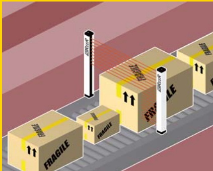
Measurement of the height of objects in transit on conveyor systems
