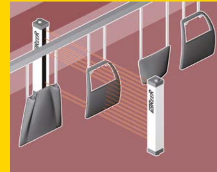
Detection of position and profile of pieces in automatic painting systems
